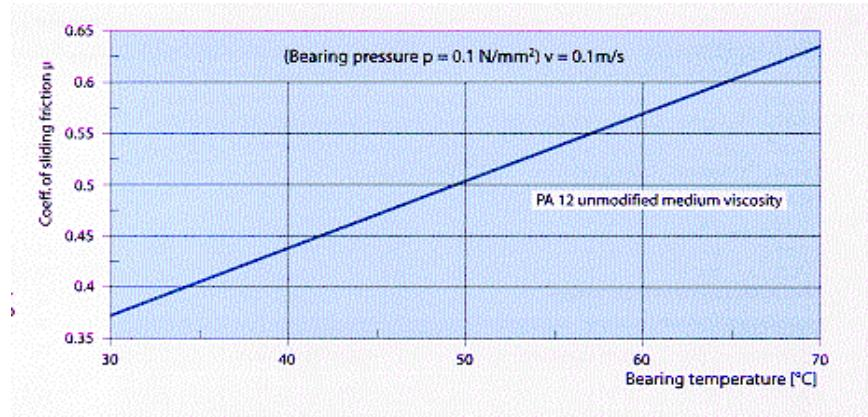
Coefficient of sliding friction in dependence of bearing temperature
