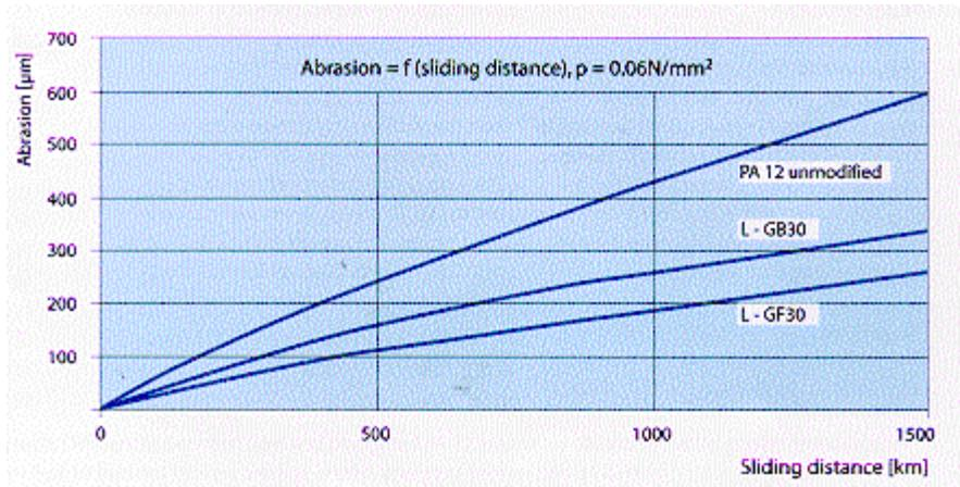
Abrasion on bearing as function of the sliding distance
