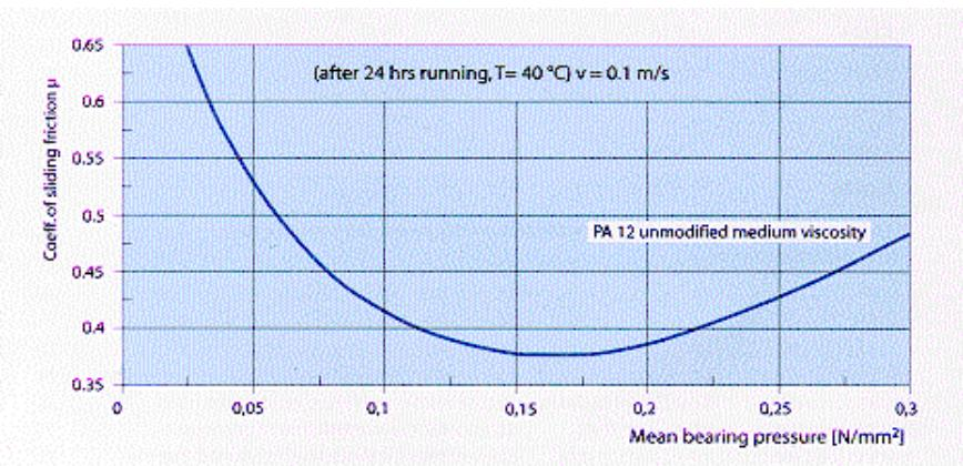
Coefficient of sliding friction as function of pressure load
